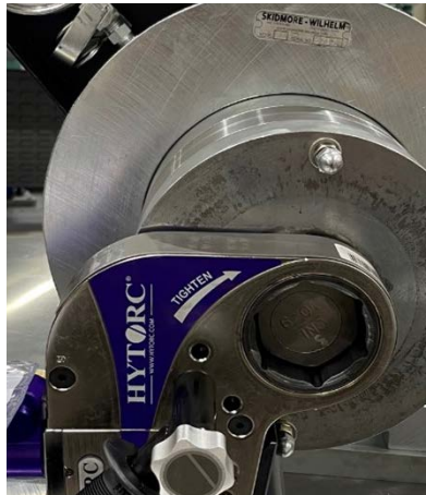
Calibrated STEALTH 4 Hydraulic Torque Wrench connected to HHCS M36 in Skidmore-Wilhelm Model K
